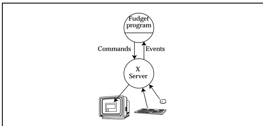
Figure 1: A Fudget program's connection with the outside world
